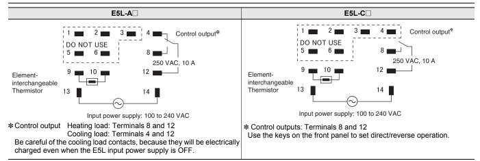
Note: For thermistor wiring, separate the input power supply and load lines as much as possible to avoid the influence of inductive noise.
