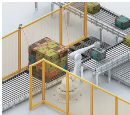
Sensing workpieces in a palletizing process
