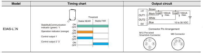
\*1. Turns off when there is insufficient margin for incident light. In that case, place the workpiece closer to ensure sufficient receiving light intensity. \*2. The initial value of control output 2 is reverse of control output 1.
