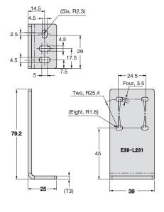
**Photoelectric Sensor** Accessory are installed (Example of E3AS-HL500□)
