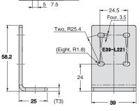
**Photoelectric Sensor** Accessory are installed (Example of E3AS-HL500□)
