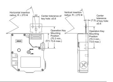
D4JL + D4JL-K2 (with Front-inserted Operation Key)
