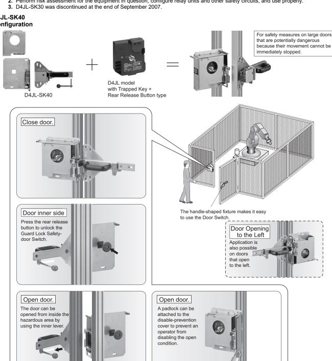
Note: This example shows a D4JL Switch with a trapped key and rear release button (D4JL-DDD-DD-DD-SJ).
