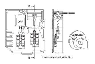
(6) Operation Key removed, solenoid ON, and trapped key
