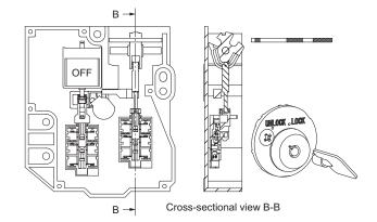
(4) Operation Key inserted, solenoid ON, and trapped key inserted. Status: Door locked and trapped key can be removed.
