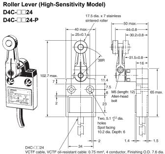
VCTF cable, VCTF oil-resistant cable: 0.75 mm², 4 conductor, Finishing O.D. 7.6 dia. SJT(O) cable: 0.83 mm², 4 conductor, Finishing O.D. 8.6 dia. D4C-I24-P (Weather-resistant Models)
