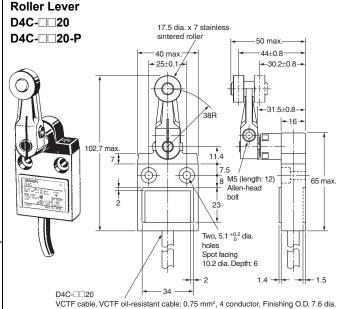
SJT(O) cable: 0.83 mm², 4 conductor, Finishing O.D. 8.6 dia. D4C-□□20-P (Weather-resistant Models)
