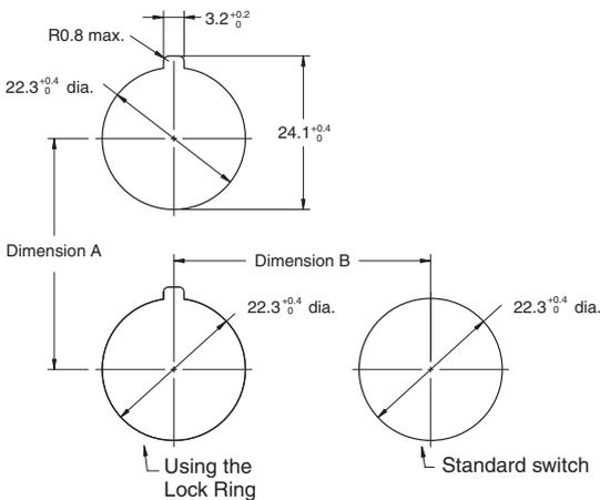
(3) Mounting the Operation Unit on the Panel
