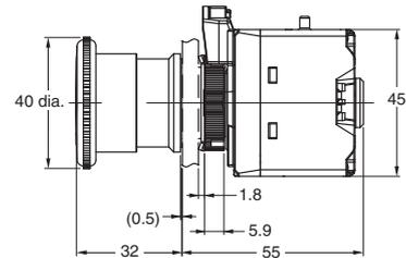
Note: The dimensions the same even if the Operation Unit is replaced with the A22NE-MR□□-N or the A22NE-MR□□-N-RD.
