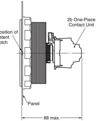
\* These are the dimension from the front of the panel when the Switch Unit is attached.
