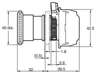
Dimensions when a two-contact Switch Block is attached
