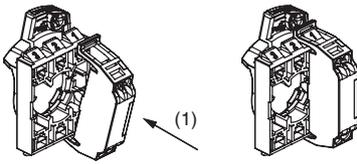
**(2) Removing the Switch Blocks and Lighting Units**
