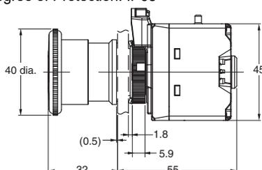
Note: Unless otherwise specified, a tolerance of ±0.8mm applies to all dimensions.
