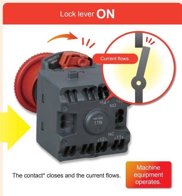
\* The example shows an NC contact. However, all contacts are interlocked with the lock lever, and the statuses of NO contacts are also switched.
