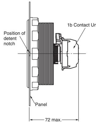
**Push-in Plus Terminal Block Type Mounting a 2-pole Switch Unit \***
