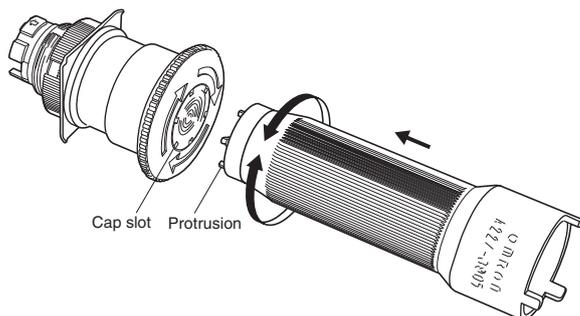
**Installing/Replacing the LED Lamp**
