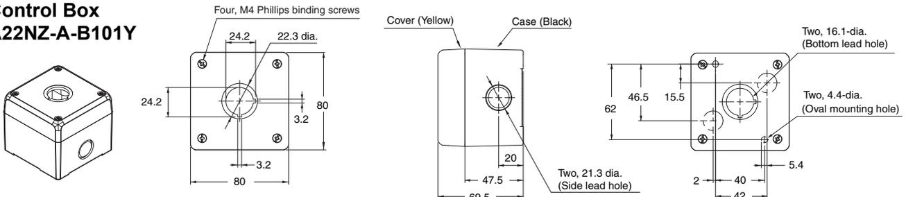
**Note:** For details on the accessories common to the screw terminal block types and push-in plus terminal block types, refer to "Common Accessories and Tools (Order Separately)" on page 51.
