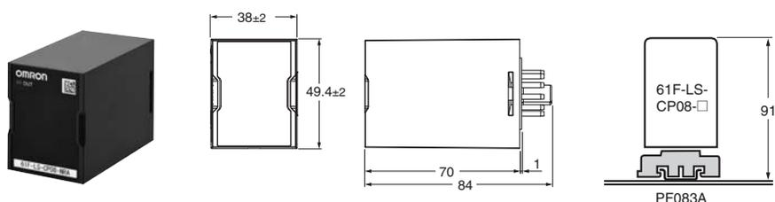
Use a PFC-N8 Mounting Bracket to mount the Level Controller to a PF083A Rail-mounted Socket.
