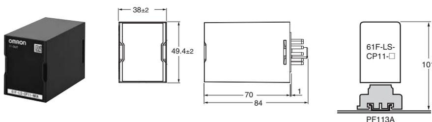
Use a PFC-N8 Mounting Bracket to mount the Level Controller to a PF113A Rail-mounted Socket.
