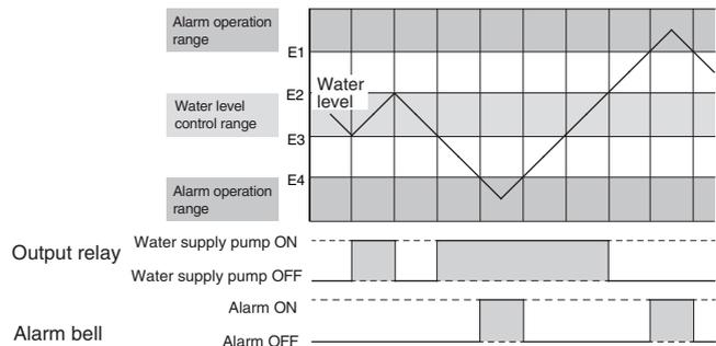
Automatic Water Supply and Drainage Control
