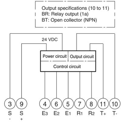
**Note:** Output is inverted when 7 and 8 are short-circuited.
