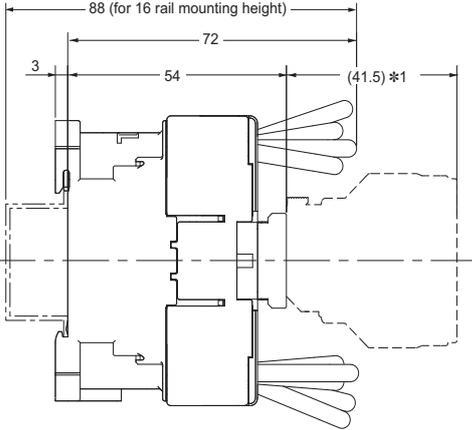
\*1. When auxiliary contact unit (J73KC) is mounted
