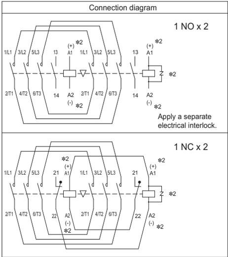
Note: The terminal (number) names of the reversing magnetic contactor are the same as the magnetic contactor.
