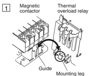
Insert the mounting legs of the thermal overload relay into the guides in the magnetic contactor, and insert the connecting wires into the terminal (insertion) holes.
