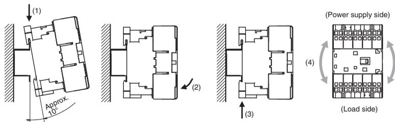
When mounting on a rail, use the end plate.
