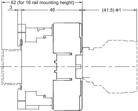
\*1. When auxiliary contact unit (J73KC) is mounted
