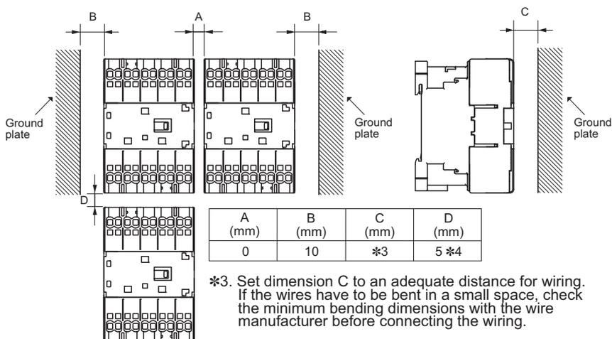
\*3. Set dimension C to an adequate distance for wiring. If the wires have to be bent in a small space, check the minimum bending dimensions with the wire manufacturer before connecting the wiring.
