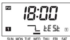
2. Press **WRITE**. The display shows the time of the next change in output state. Each time **WRITE** is pressed, the display shows the days and times for one week.
