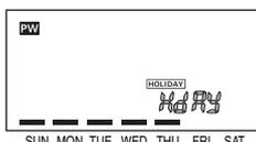
3. Press **[WRITE]** to enter the setting. After "HdRy" is displayed for approximately 1 s, the Time Switch returns to RUN mode.
