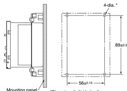
\*Diameter of pilot holes for included M4 tapping screws (guideline)
