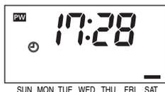
4. Press **[WRITE]** to enter the setting, and the Time Switch will start from 0 second.
