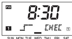
2. Press **WRITE**. The display shows the time of the next change in output state.
