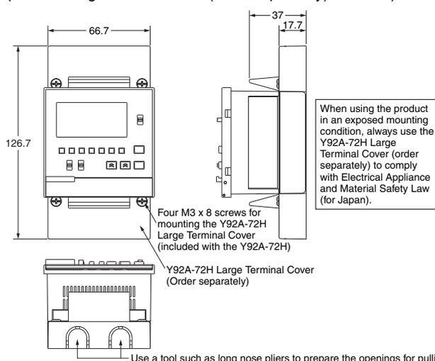
When using the product in an exposed mounting condition, always use the Y92A-72H Large Terminal Cover (order separately) to comply with Electrical Appliance and Material Safety Law (for Japan).
