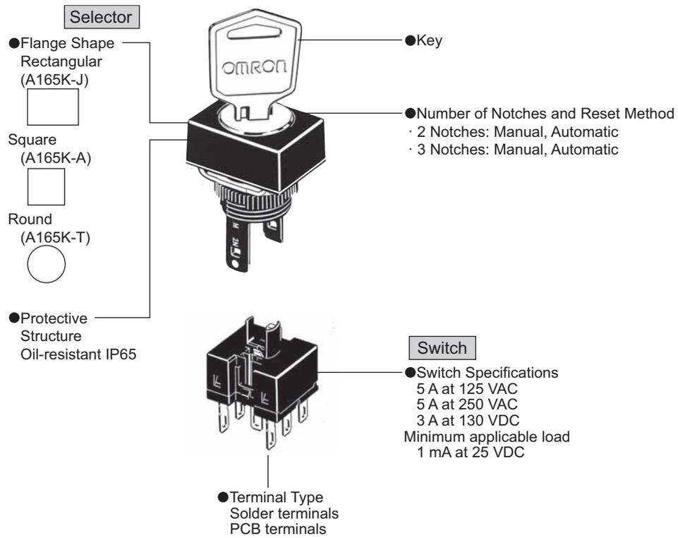
**The flange can be rotated to easily change the operation angle of the knob.**
