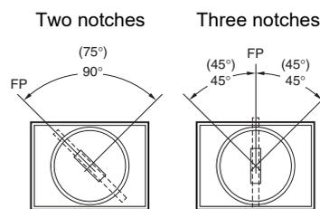
Note: The angle used for automatic reset is shown in parentheses.
