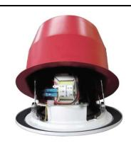
This voice alarm ceiling loudspeaker is specifically designed for use in buildings where performance of systems for voice evacuation announcements is governed by regulations. It is designed for flush in suspended ceiling and ideal for even sound distribution. The appearance and neutral white RAL 9003 color have been selected to be unobtrusive in virtually all interiors. The fire dome increases protection of the cable termination.
