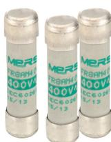
Mersen aM and gG fuse-links cover a wide range of physical sizes and ampere ratings for 400, 500, and 690VAC for protection in electrical distribution circuits and various industrial applications. Most ratings are available in size 8x31 and size 10x38 with an optional indicator, and in size 14x51 and 22x58 with an optional striker to activate an auxiliary contact. Size 10x38 is also available with striker. All cylindrical fuse-links have ceramic bodies and silver-plated contacts.
