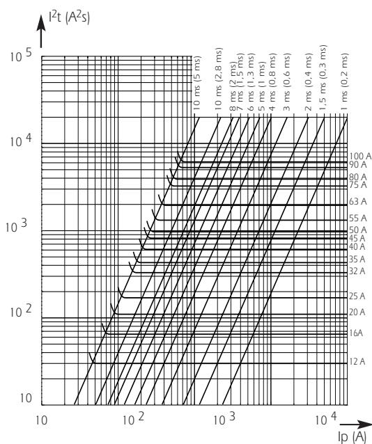
Above: Horizontal curves show for each rated current maximum values of total clearing  $I^2t$  ( $I^2t_t$ ) as a function of prospective current  $I_p$ , @ 690 V.
