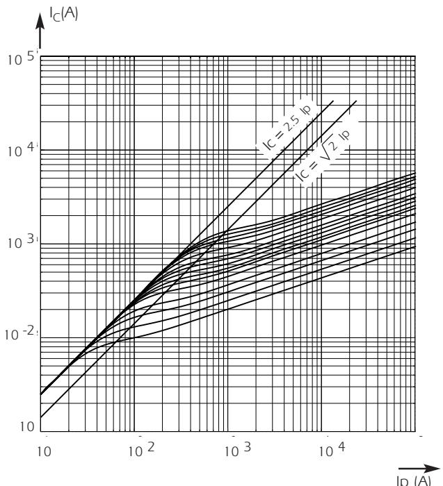
Above: Curves show, for each rating, value of peak let-through current  $I_C$  as a function of available fault current  $I_p$ .
