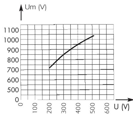
Curve indicates peak arc voltage  $U_m$  which may appear across the fuse terminals at working voltage  $U$ .
