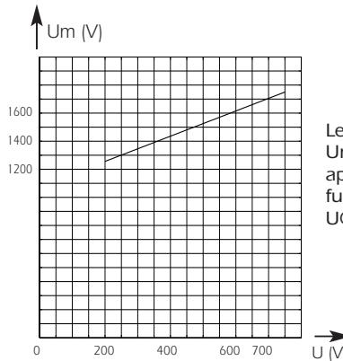
Left: Curve shows peak value  $U_m$  of arc voltage which appears across fuse-link as a function of operating voltage  $U$  @  $\cos \varphi = 0.15$
