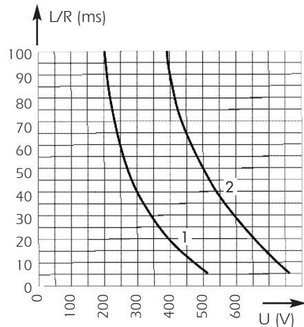
Above: Curves indicate permissible value of time constant L/R as a function of DC working voltage.
