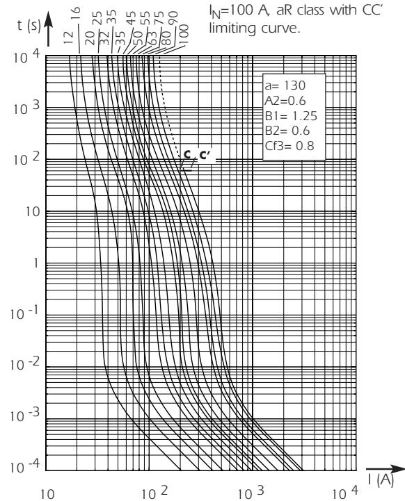
Tolerance for mean pre-arc current ± 9%.
