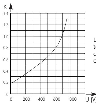
Left: Curve shows variation of total clearing time ( $I^2t_t$ ) and total clearing duration  $T_t$  as a function of operating voltage  $U$ .
