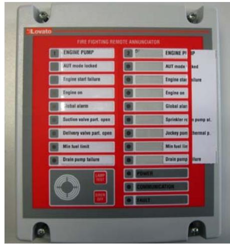
Divide the labels on the die cut lines and insert them into their housing on the front panel:
