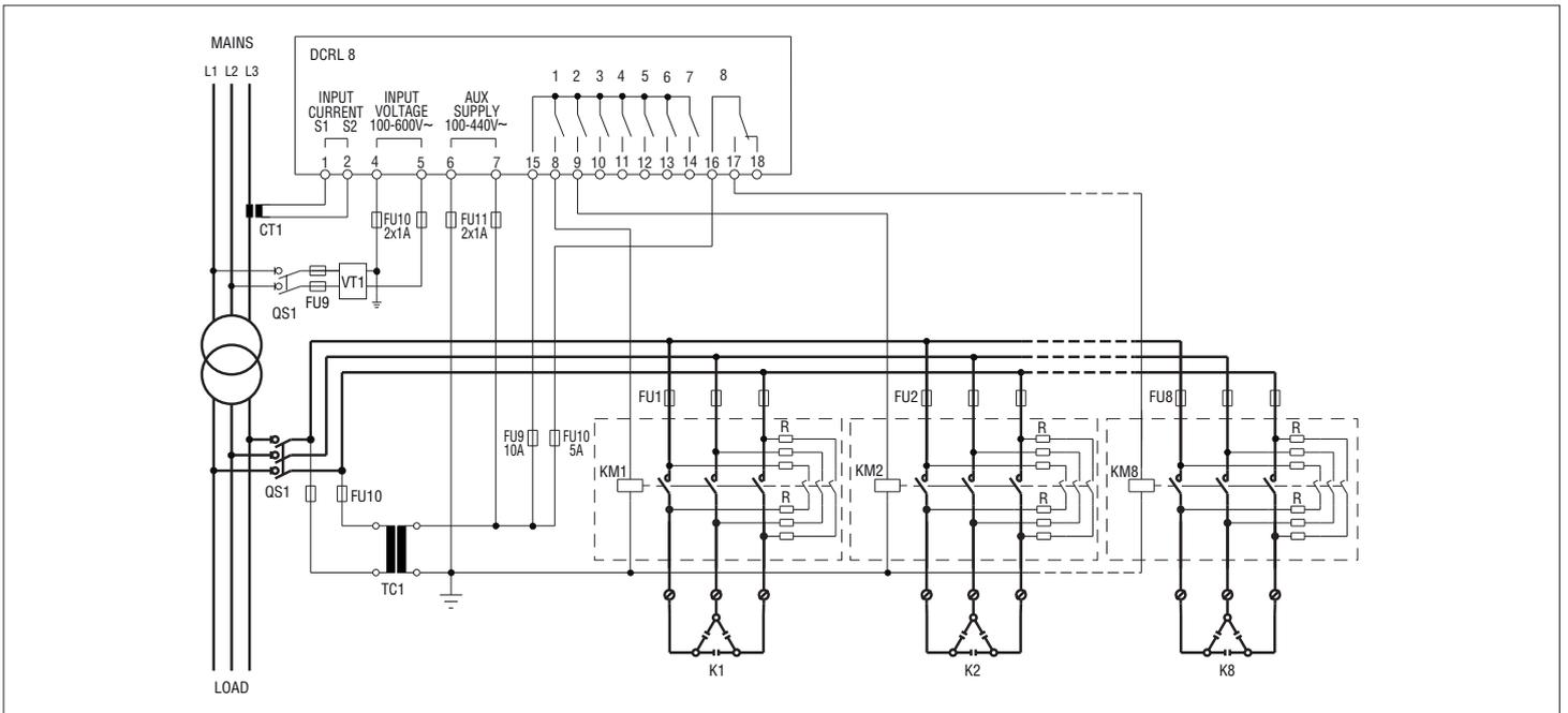
Configuration with MV measurement and correction
