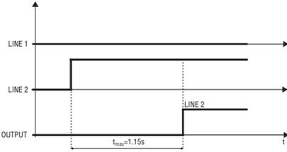
Maximum switching time upon connection of Line 1 with Line 2 present.
