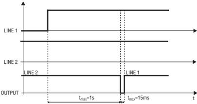
Maximum switching time upon disconnection of Line 1 with Line 2 present.
