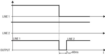
Maximum switching time upon simultaneous connection of Line 1 and Line 2.
