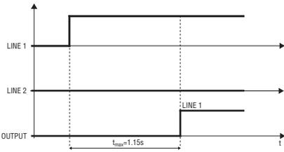
Maximum switching time upon connection of Line 2 with Line 1 absent 1.15 sec
