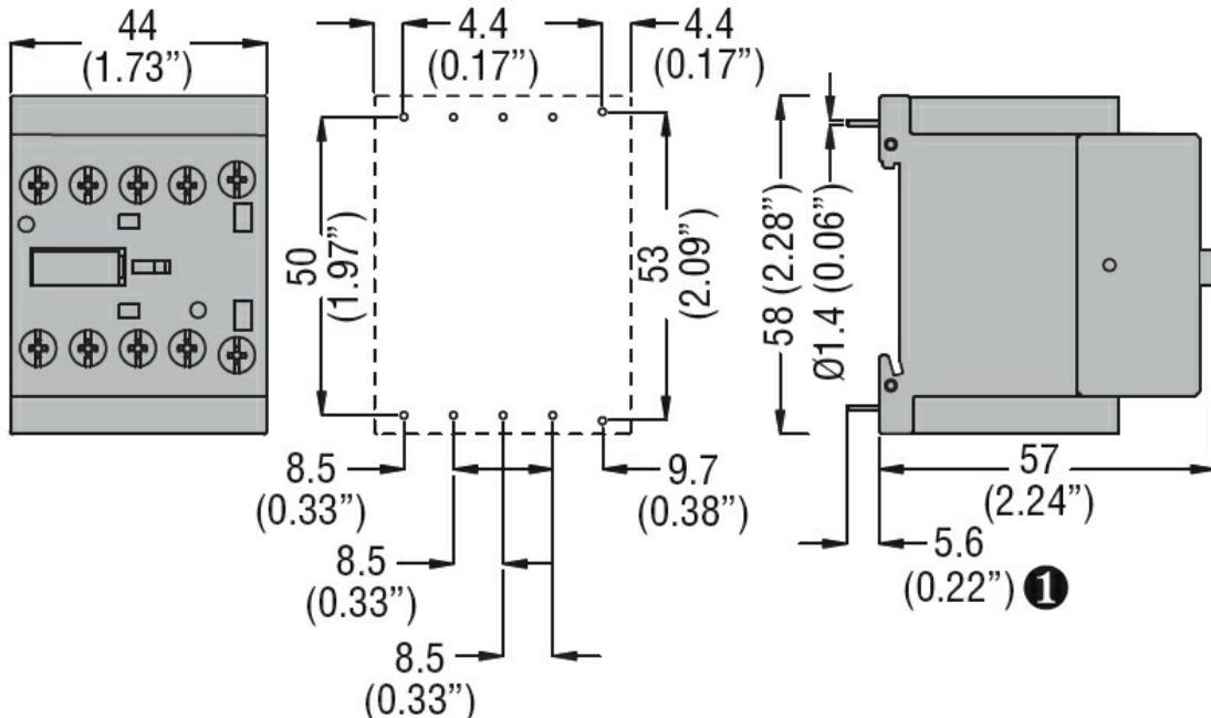
**①** Recommended PCB drillings 1.7-2mm.
