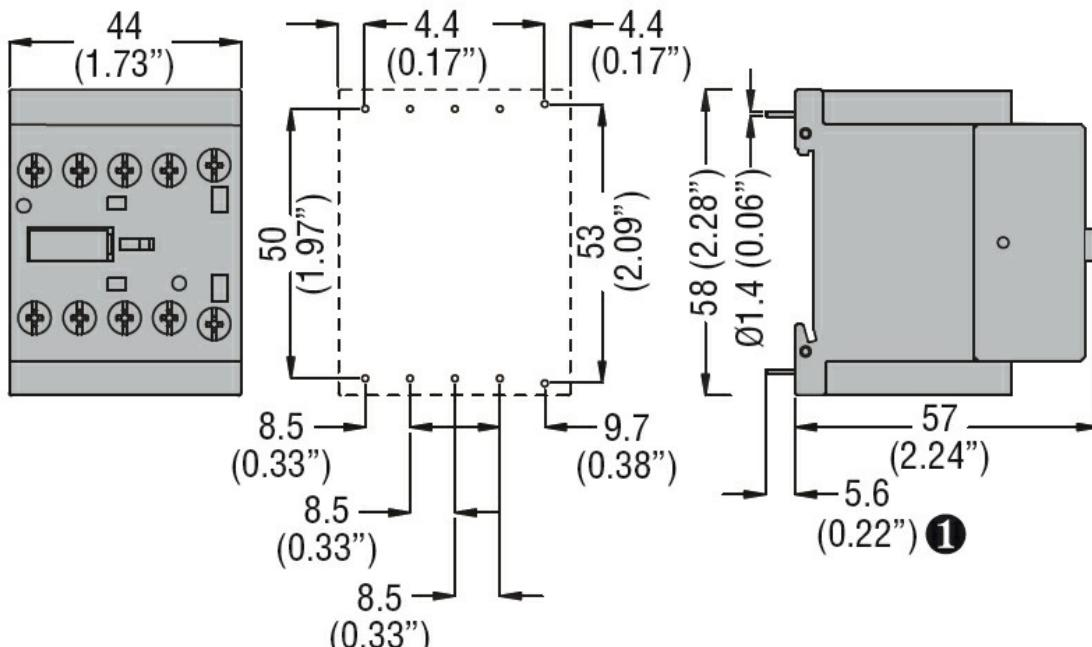
① Recommended PCB drillings 1.7-2mm.
