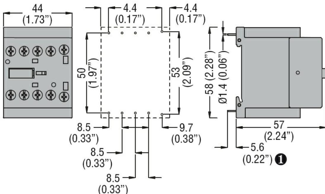
**①** Recommended PCB drillings 1.7-2mm.
