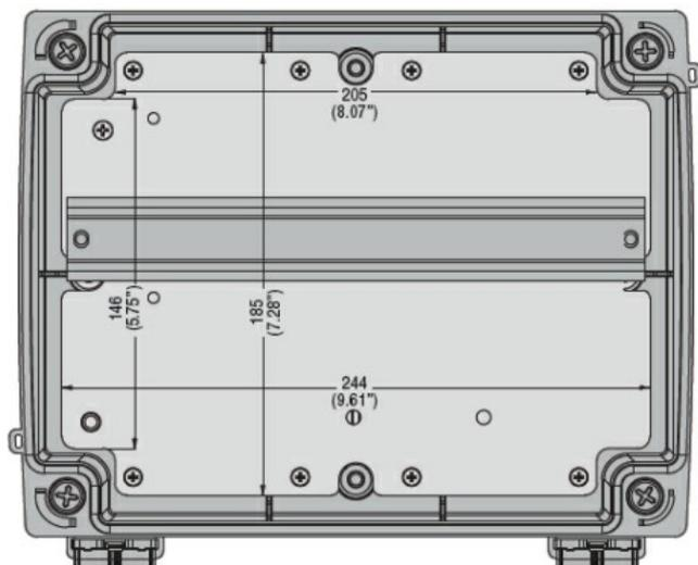
Drilling for surface fixing
