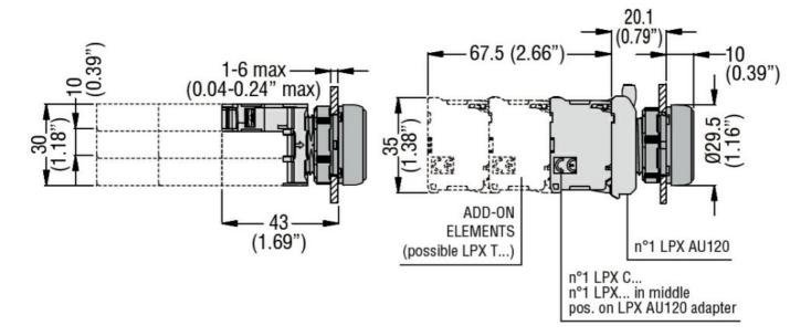
LED INTEGRATED LAMP-HOLDER, STEADY LIGHT Ø22MM PLATINUM SERIES, SCREW TERMINATION, 12...30VAC/DC. BLUE
