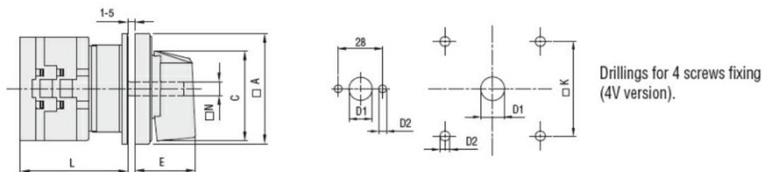
Drillings for 4 screws fixing
