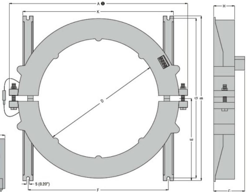
● With screws, for RTA210 split-core type; fixed structure, without screws, for RT210 type.
