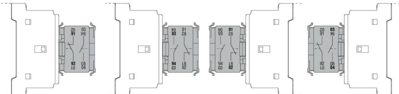
The termination of the G218 auxiliary contact has more than one numbering due to the fact that the block can assume various mounting positions. See the numbering in boldface for a correct interpretation.
