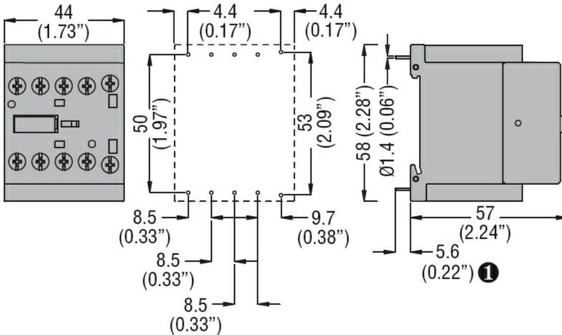
① Recommended PCB drillings 1.7-2mm.
