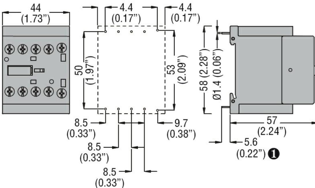
① Recommended PCB drillings 1.7-2mm.
