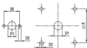
Drillings for 4 screws fixing
