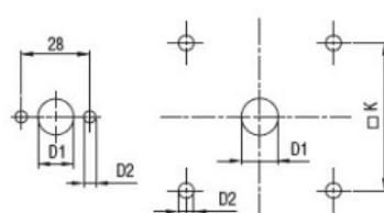
Drillings for 4 screws fixing (4V version).
