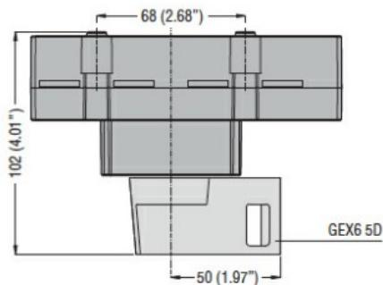
With terminal cover and auxiliary contact
