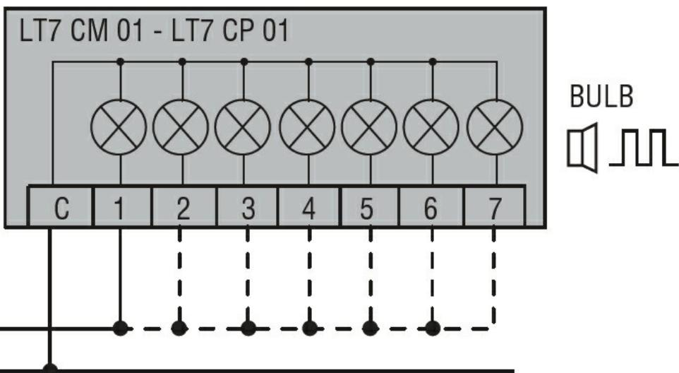
Connect terminals C and 1 as indicated to power the first module.
