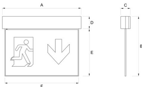
A=271mm B=206mm C=33mm D=43mm E=163mm F=255mm
