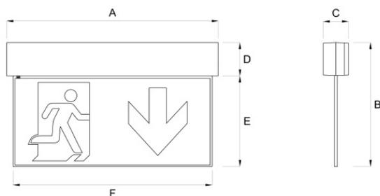
A=271mm B=167mm C=33mm D=43mm E=123mm F=255mm
