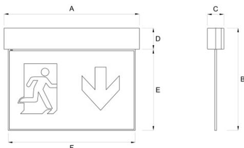
A=271mm B=206mm C=33mm D=43mm E=163mm F=255mm
