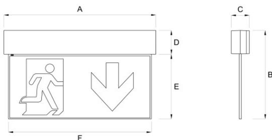
A=271mm B=167mm C=33mm D=43mm E=123mm F=255mm
