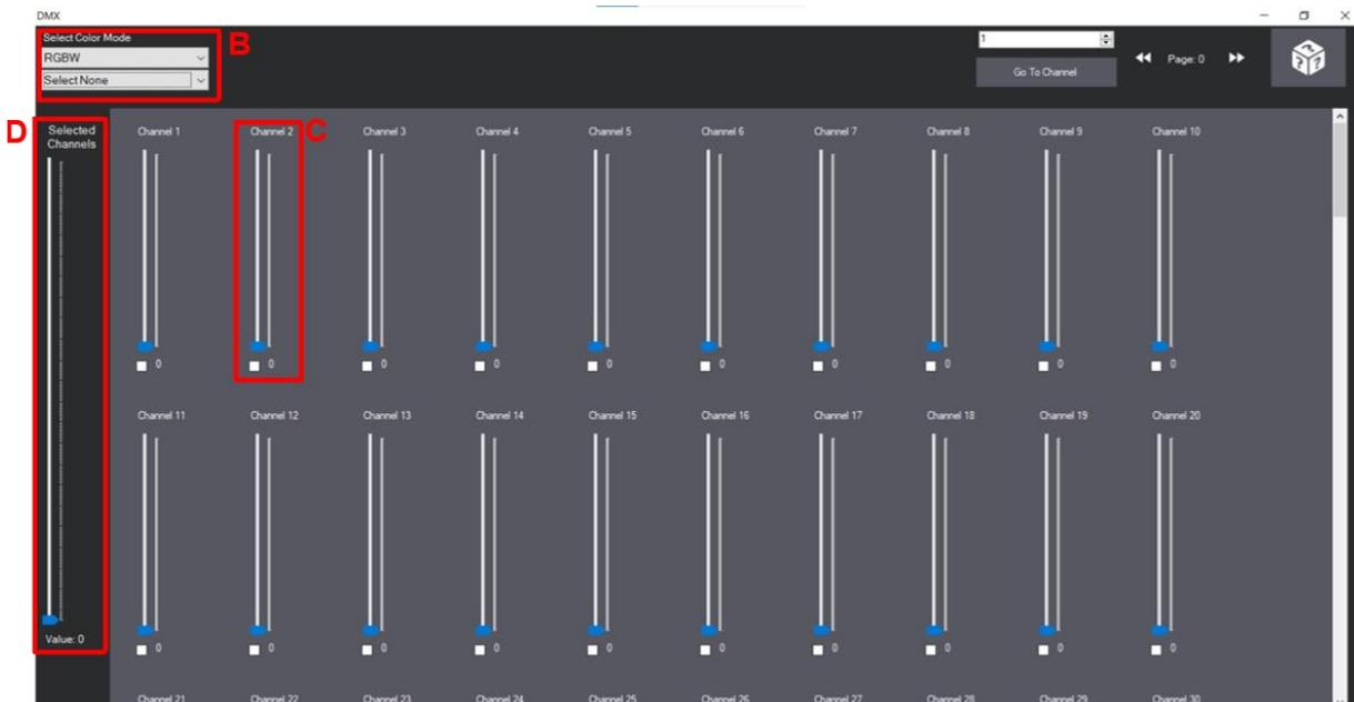
2) Using the sliders, it is possible to control individual channels from 1 to 512.
