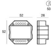
Dimmer - RF Remote Control - 12-48V 4CH WIFI-PUSH-TEL per Ribbon Plus, Ribbon PRO, Ribbon PRO 48V, PU\_C, Rubber 2D Mini, Rubber 3D, Rubber 3D PROtection, Rubber 3D Concrete, Rubber 3D 48V, Rubber 3D OPTIC RF Remote controller
