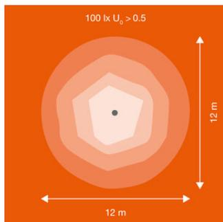
Floodlight Performance 150W SYM 60 simplified isolux diagram
