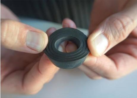
SKINDICHT® Incised sealing rings can be customized for individual cable diameters. Therefore the inner single layers can be cut off with a knife step by step.
