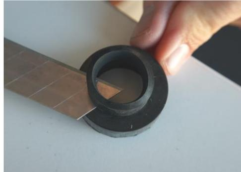
Further the cutter should gently be pressed into the connector film, and then cut slowly clockwise until the inner ring is cut out.
