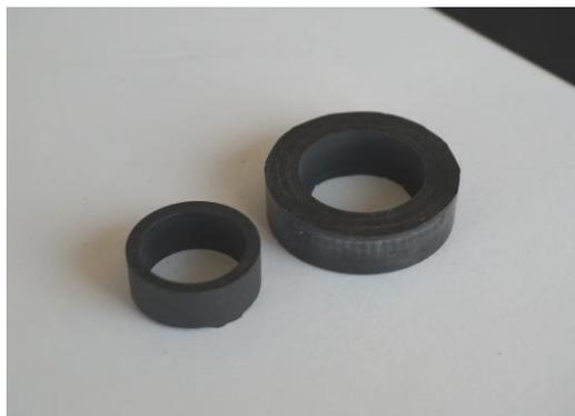
The picture shows the prepared incised sealing ring for the cable installation (right side). Repeat process 2 and 3 until the cable diameter fits in the clamping range of the incised sealing ring.
