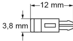
**CDSH series - Coding with CR CDS pins**
