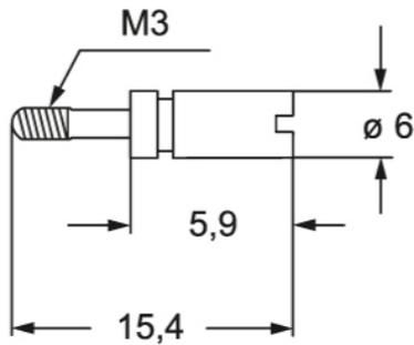
Coding options using the three coding and guiding pins
