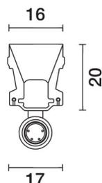
versione Top-Bend 16mm - Led Neutral white - High output - 24Vdc - L= 7004mm
