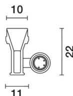
versione Side-Bend 10mm - Led Neutral white - 24Vdc - L= 1004mm
