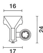
versione Side-Bend 16mm - Led Warm white -24Vdc - L= 254mm
