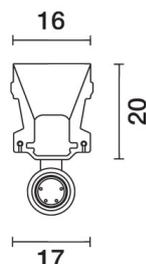
versione Top-Bend 16mm - Led Neutral white -24Vdc - L= 2004mm
