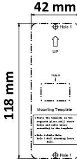
Figure 2-2 Mounting Template
