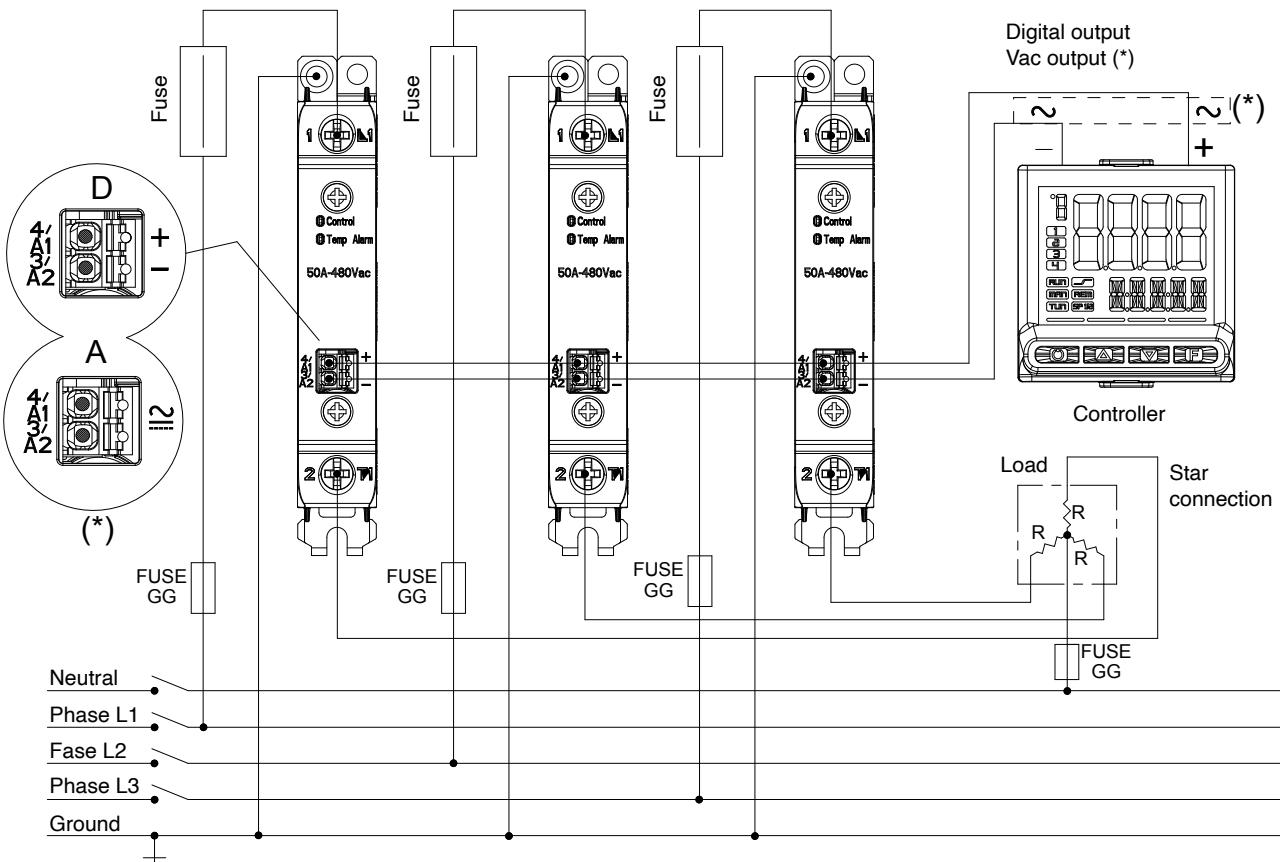
(\*) Or relè output with Vac tension (Use grs-h with command input Vac type a)
