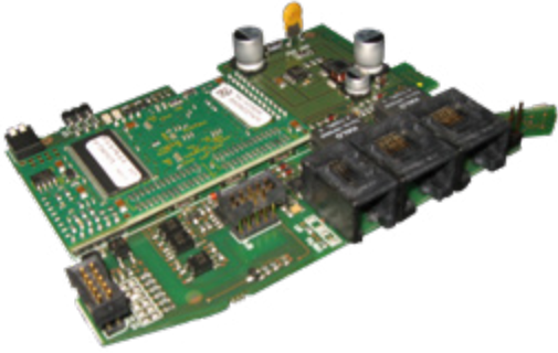
Figura 36 Port2: Interfaccia Modbus RTU / Ethernet IP o Modbus RTU/EtherCAT o Modbus RTU / ProfiNET
