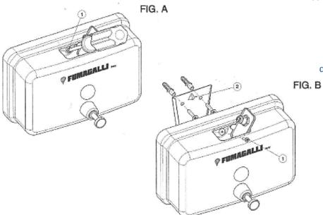
Fix bracket N° 2 to the wall using the dowels and the screws provided. Insert the soap dispenser in the soap dispenser guide and fasten it using screw N° 1 as shown in figure B.
