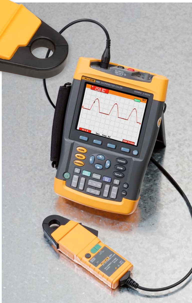
i30s collegata a uno ScopeMeter™ Fluke 199C
