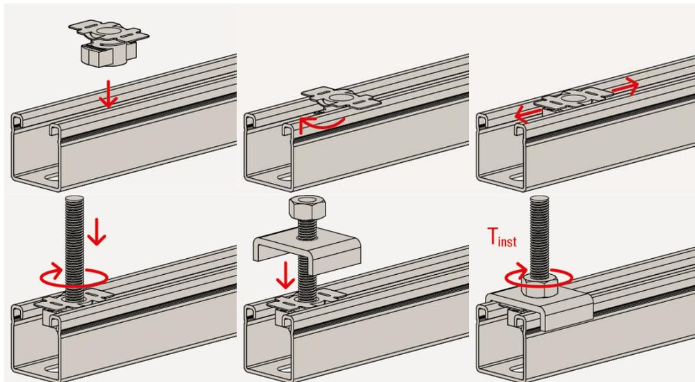
Table B 2.2 shows the installation torques  $T_{inst}$  for the installation of the saddle nut FCN Clix P in combination with the drilled plate HK 41 and a threaded rod of property class 4.8 or higher with the FUS channel system depending on the thread size.
